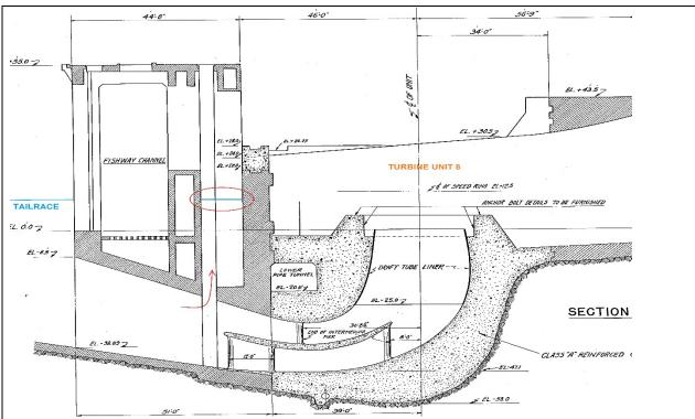
**Figure 1.** Schematic of the PH1 turbine outflow area. The tailrace is to the left and the forebay to the right. The suspected point of entry of fish into the area described is denoted as the red arrow. The dead fish were noted in the location of the red circle. Unit 8 has been out of service with no flow or tail logs since 22 February 2016.
